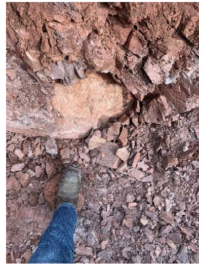
Figure 2 - Weathered rock that is diggable.
